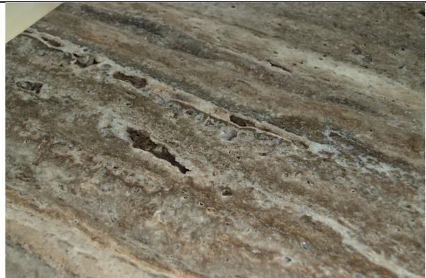
EXAMPLE OF HOLES FILLED WITH RESIN
