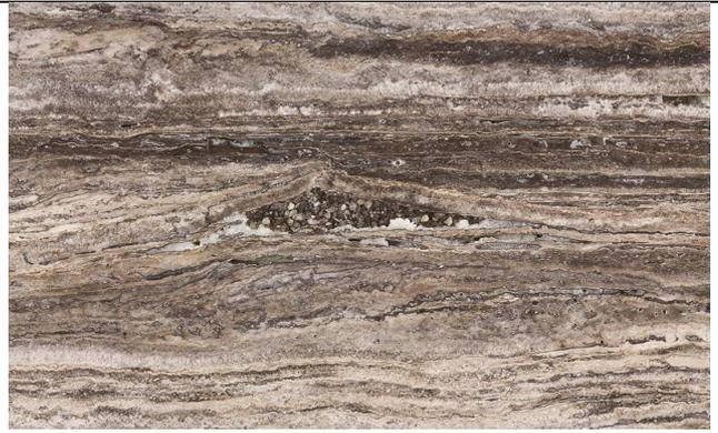
EXAMPLE OF NATURAL HOLE FILLED WITH RESIN AND SMALL TRAVERTINE GRAINS
