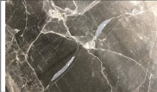
EXAMPLE OF NATURAL HOLES FILLED WITH RESIN - 1
